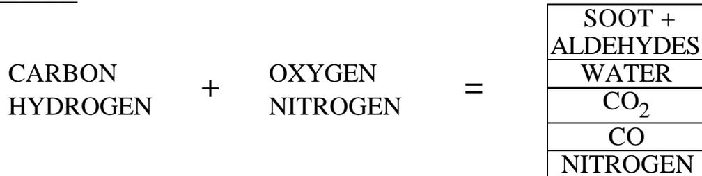
Perfect combustion (stoichiometric combustion) is the process of burning the fuel without an excess of combustion air. This process should develop the “ULTIMATE CO<sub>2</sub>” amounts in the combustion products.
